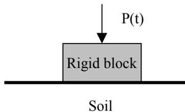
If we assume the soil as linear then the impulse response may be obtained (albeit approximately) by subjecting the area where the block rests to a load that grows and decays very quickly (through a rigid lightweight plate). If we take the Fourier Transform of the impulse response we obtain a frequency response function which can be expressed as;
