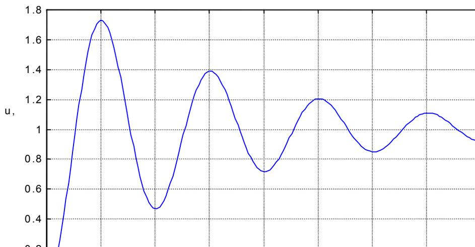
The solution for a step load where  $\Delta_{st}=1$  is illustrated in Figure 1. In this case, the damping is 10% and we see that the peak is approximately equal to 1.78. It can be shown that if the damping is zero, the peak would be  $2*\Delta_{st}$  (See Figure 2). Therefore damping is not that efficient in reducing the response for a step load. This is generally true when the maximum response occurs early.
