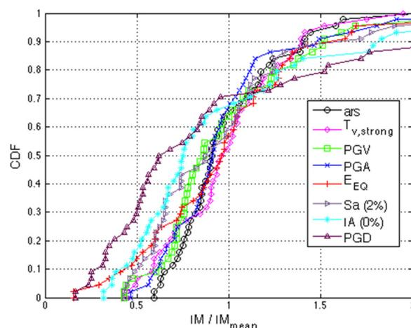
Figure 8. Cumulative distribution function of IM-collapse level for the test case of Lignos et al. (2008) subjected to ATC-63 far field record set (44 ground motions).
