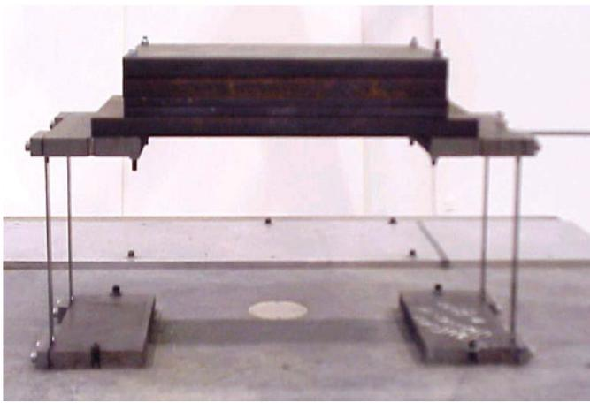
Figure 1. Specimen configuration (Kanvinde 2003).
