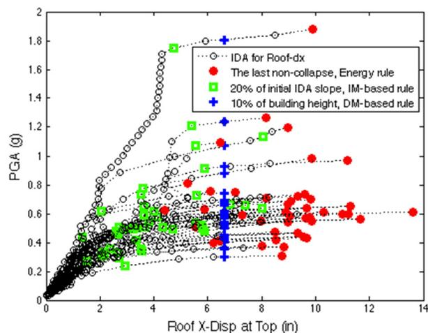
Figure 7. IDA curves and comparison of collapse criteria for the test case of Lignos et al. (2008) subjected to ATC-63 far field record set (44 ground motions).
