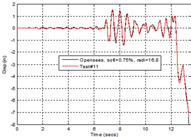
Figure 2. Displacement time history results by OpenSees for the test case by Kanvinde (2003) under the test ground motion record of the 1994 Northridge at Obregon Park. “soft” and “radi” in the plot refer to the softening amount and radius of transition from elastic to plastic branches in the springs respectively.
