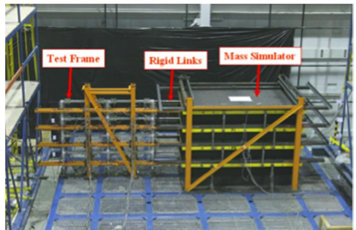
Figure 3. Shake-table-test of a 1/8 scale 4-story, 2-bay steel frame with reduced beam sections (Lignos et al. 2008).
