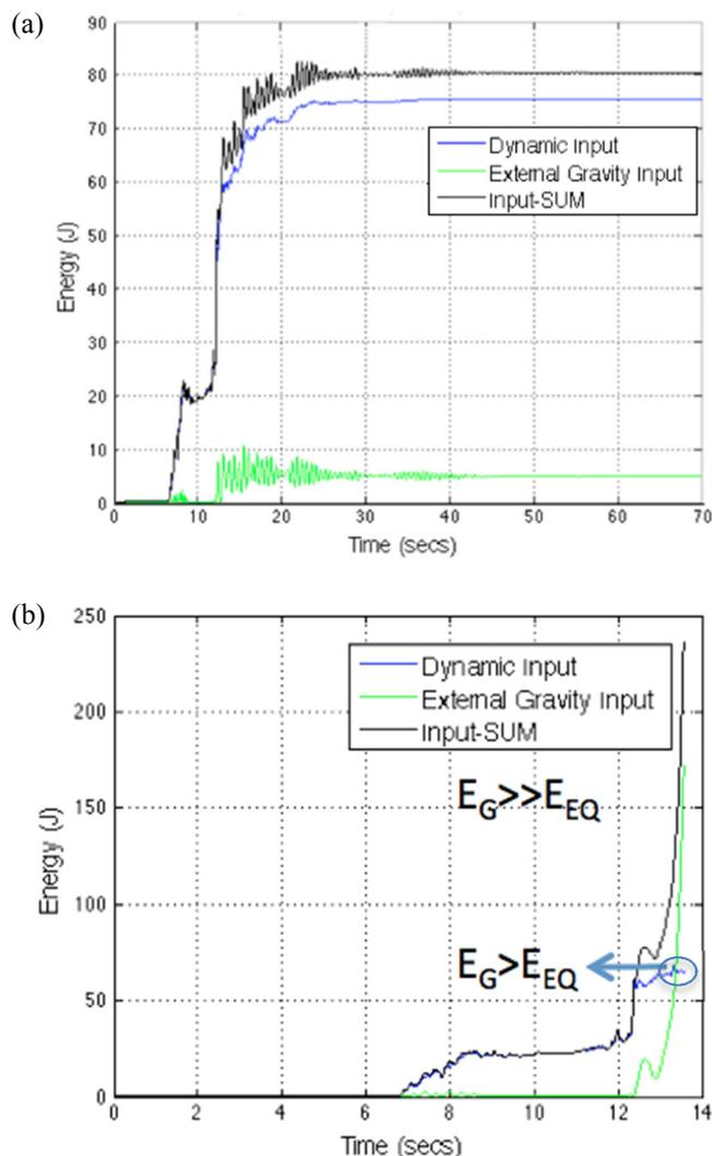
Figure 6. Input energy components near collapse under the test earthquake of 1994 Northridge earthquake at Obregon Park a) non-collapse case at the ground motion scale of 0.8 and b) collapse case at the ground motion scale of 1.0.
