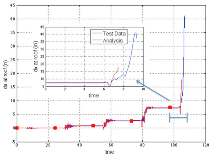
Figure 4. Comparison of experimental test results and simulation results of lateral displacement time history at the top of the frame for the test case by Lignos et al. (2008). Note that the simulation model here depends on the clear span model, and was continuously subjected to the ground motion record of the 1994 Northridge earthquake at Canoga Park with a scale factor of 0.4, 1.0, 1.5, 1.9, and 2.2 following the test procedure.
