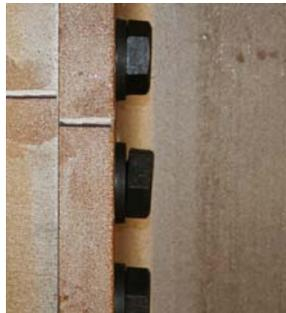
**Figure B.109 – 159n1: Bolt SE5 after slip (south side)**
