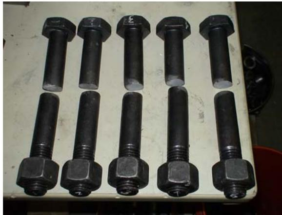
Figure 16 – Failed TN 9 in. bolts due to shear [from (Rassati and Swanson, 2007)]
