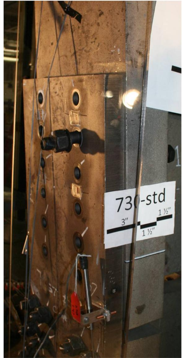
**Figure B.4 – 730-std: After test (south side)**
