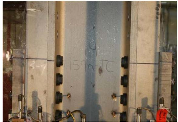
**Figure B.360 – 159n-TC: After initial slip (west side)**
