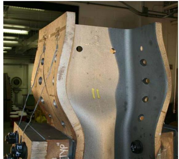
Figure B.388 – 159f-weld: After test (east side)
