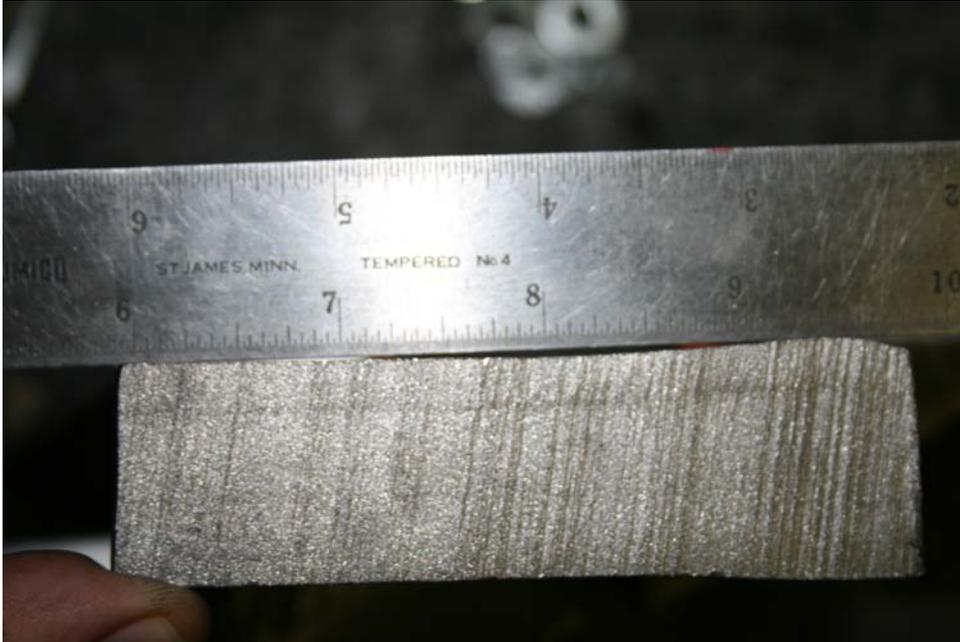
**Figure 21 – Slip specimens cut from W14x159 flange**
