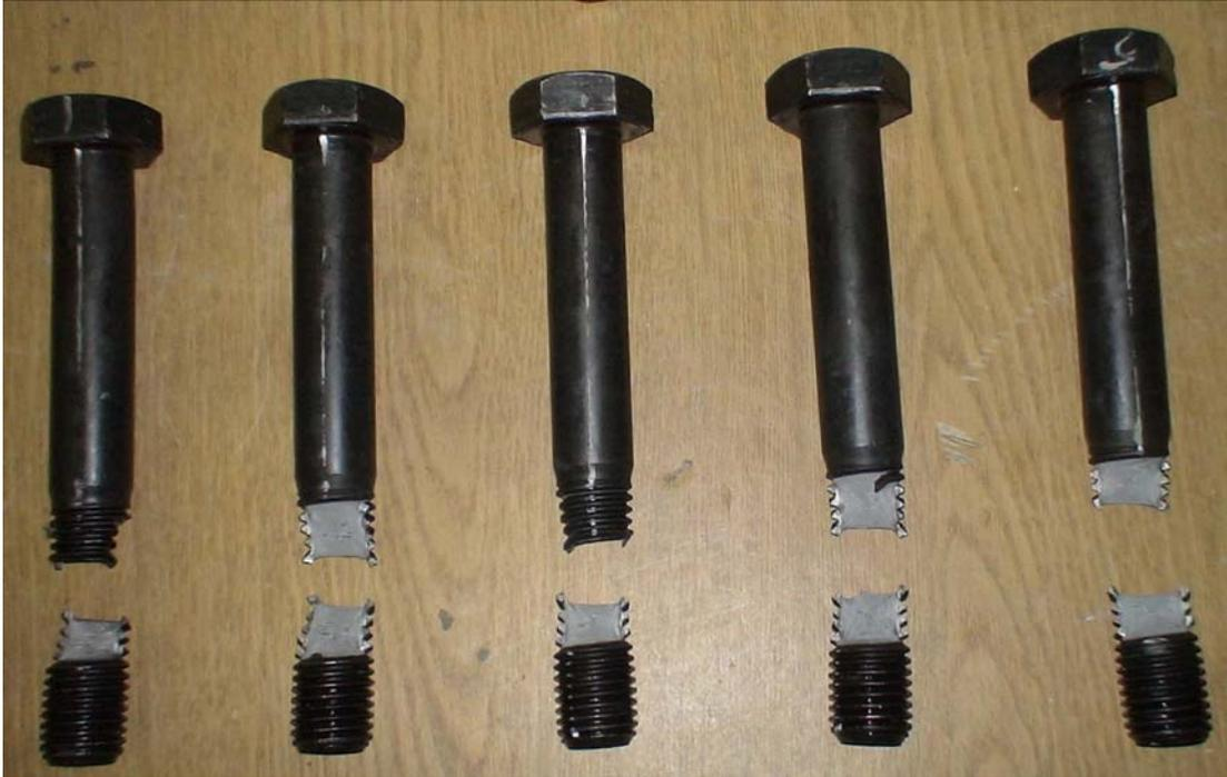
**Figure 13 – Failed TN bolts due to tension [from (Rassati and Swanson, 2007)]**
