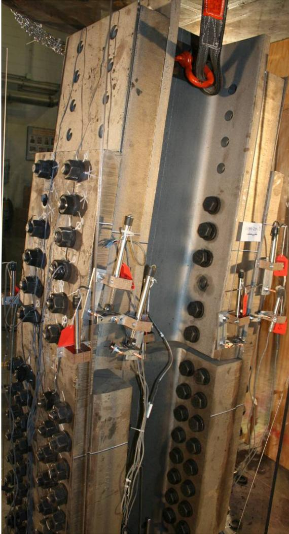
**Figure B.276 – 159n-2ply1: Initial single bolt failure (northwest corner)**
