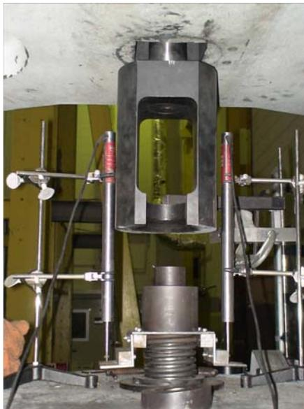
**Figure 12 – Bolt tension test apparatus [from (Rassati and Swanson, 2007)]**
