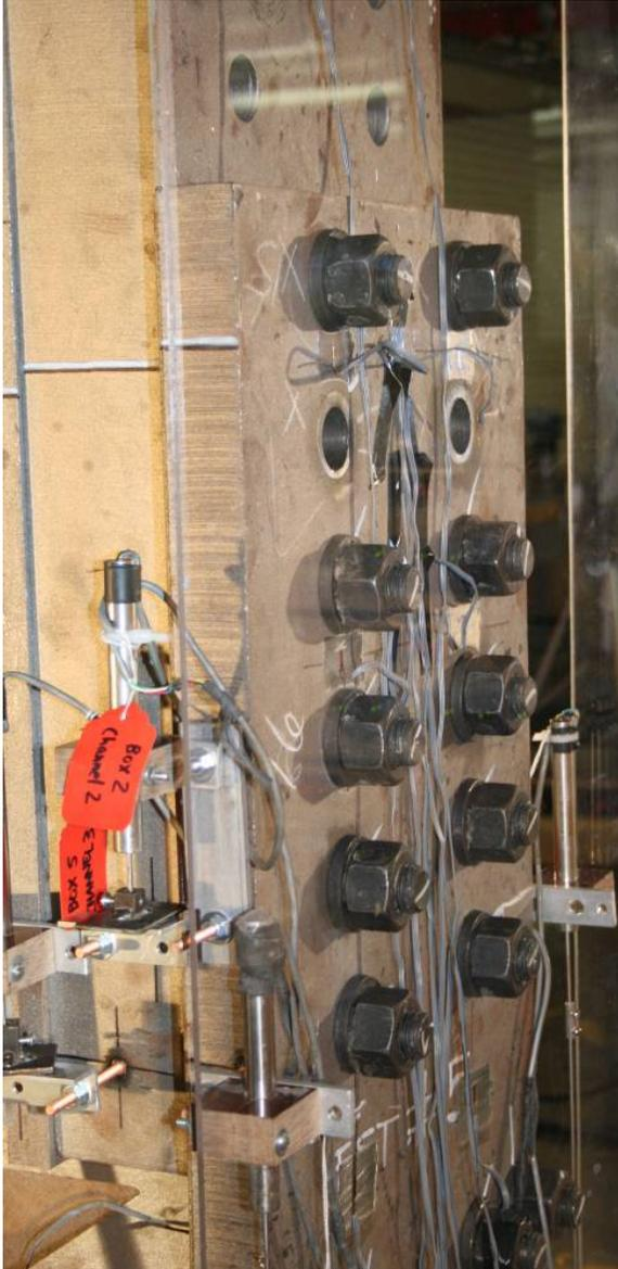
**Figure B.136 – 159n2: After slip (south side)**
