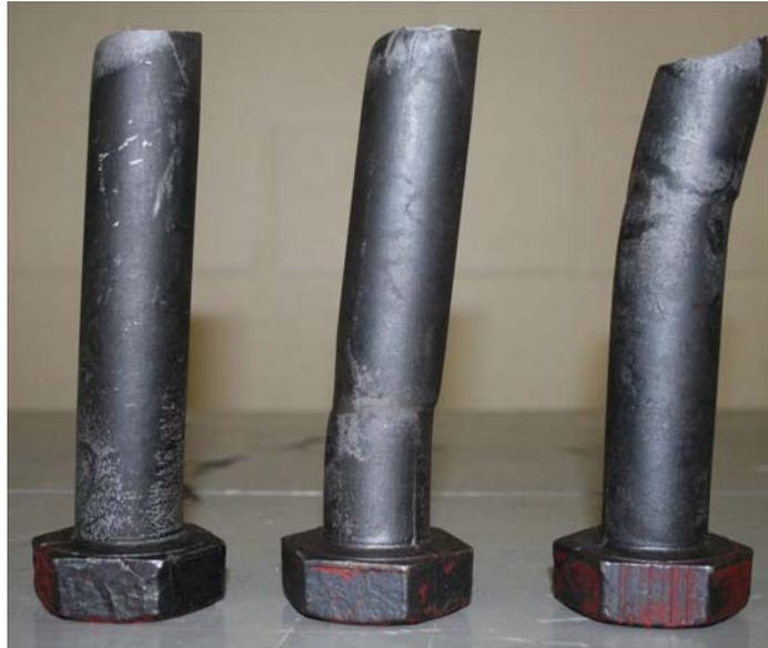
**Figure 46 – Specimen bolt deformation (730-over, 159n1, and 455n1)**
