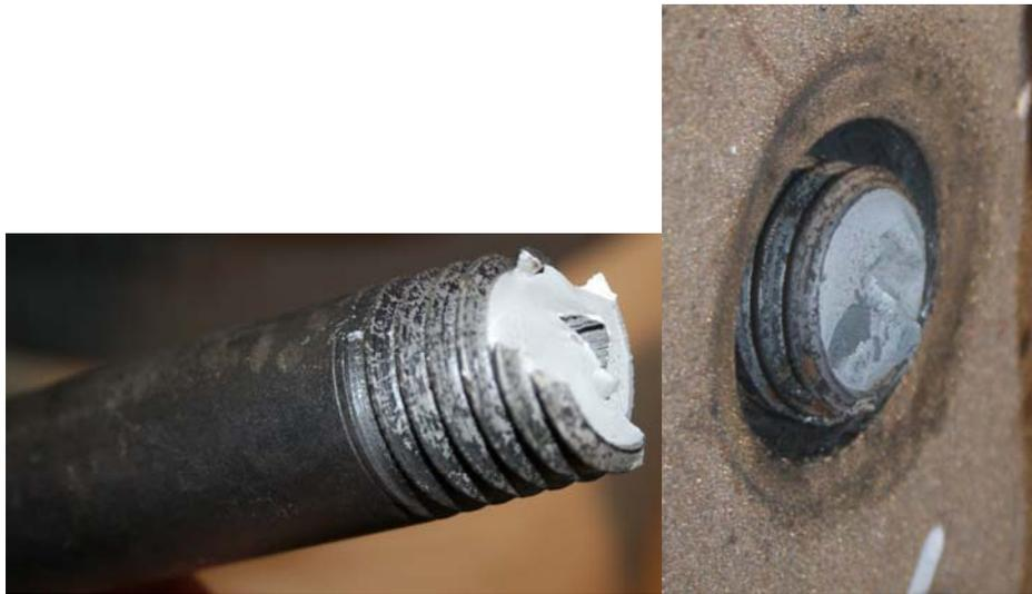
**Figure 25 – Premature bolt failure through threads**
