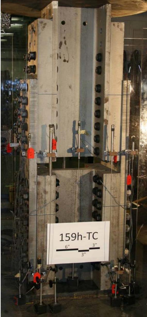
**Figure B.329 – 159h-TC: After initial slip (east side)**
