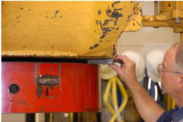
**Figure 8 – Wedge for locking loading platen**
