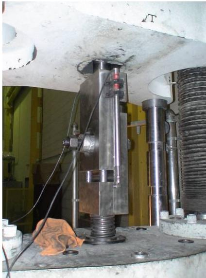
Figure 15 – Bolt shear test apparatus [from (Rassati and Swanson, 2007)]
