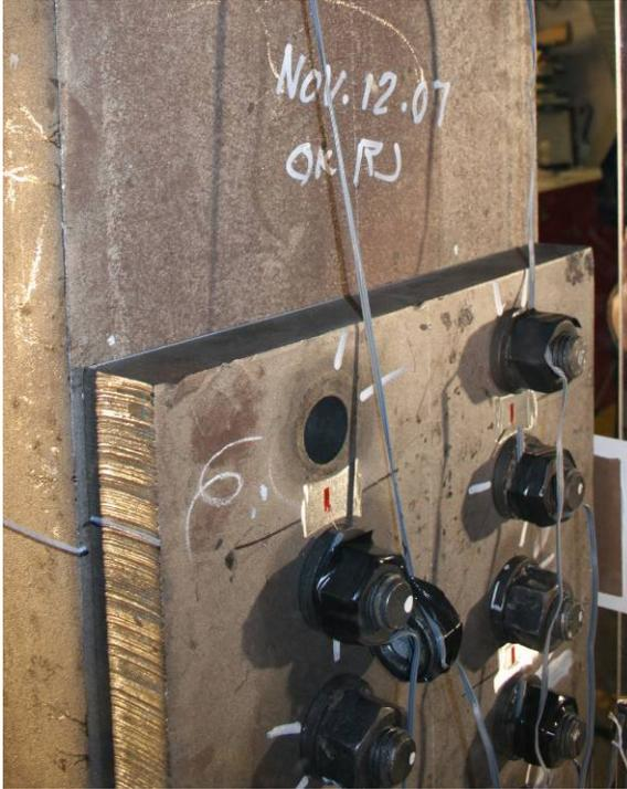
**Figure B.26 – 730-over: Early bolt failure (south side)**
