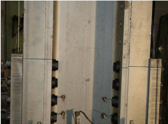
**Figure B.359 – 159n-TC: After initial slip (east side)**
