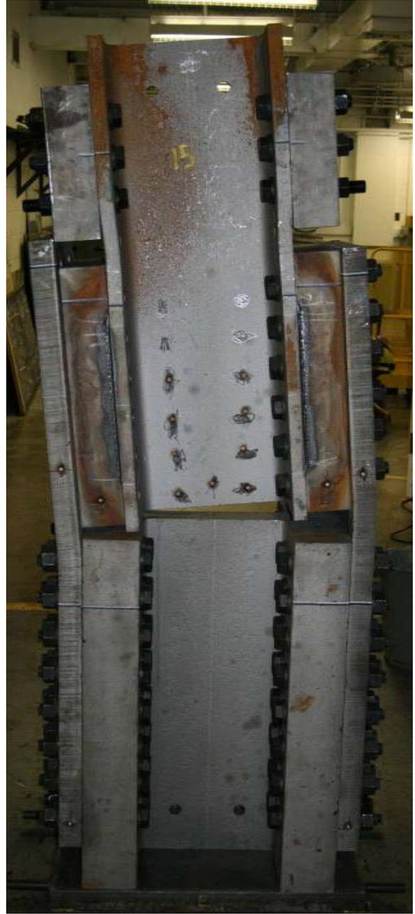
**Figure B.416 – 159h-weld: After test
