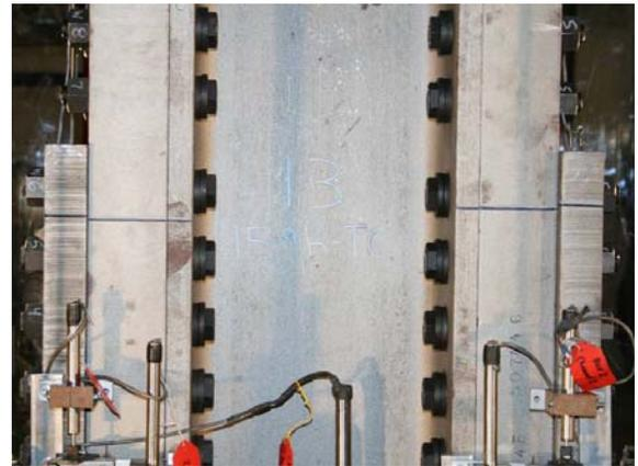
**Figure B.330 – 159h-TC: After initial slip (west side)**
