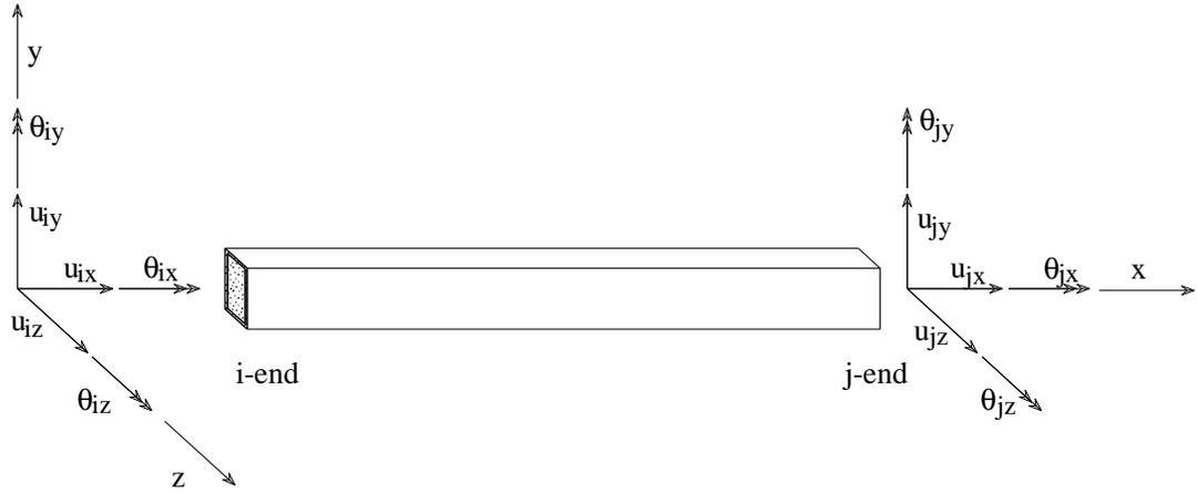
**Figure 3.2** CFT Beam Element
