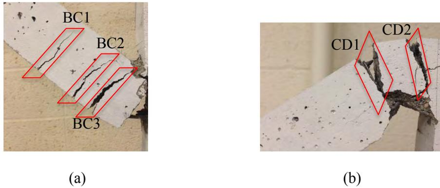
Figure 7.20: Labeled cracks for (a) BC-1-1 and (b) CD-3-1.
