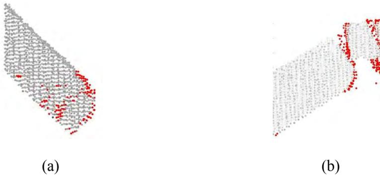
Figure 7.22: Damage detection results for  $k = 6$ , where (a) BC-1-1 ( $T_{int} = 0.63$ ) and (b) CD-3-1 ( $T_{int} = 0.78$ ).
