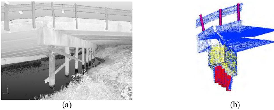
Figure 10.14: (a) Scan data of DeKalb County Bridge with section utilized for data processing, and (b) point cloud of the same section with four piers detected as cylinders and pier cap surface detected as planes.
