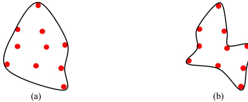
Figure 7.27: (a) Convex hull representation of a sample defect dataset and (b) actual geometric representation of the defect.
