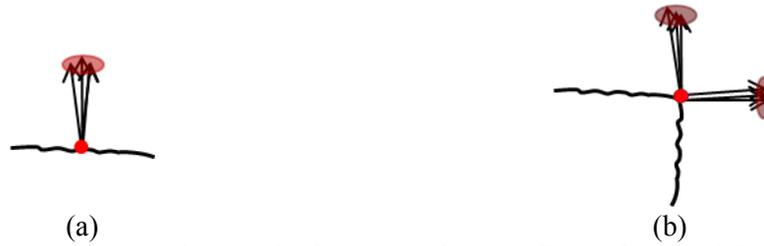
Figure 5.12: Gauss map clustering results for (a) a point on a flat surface; and (b) an edge point.
