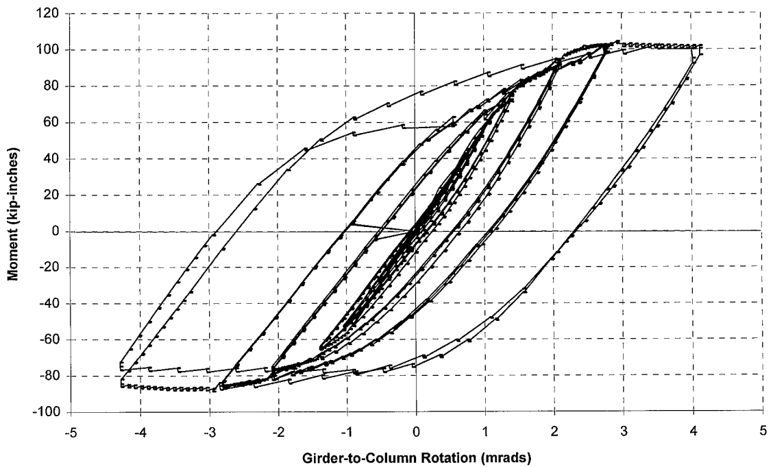
Figure B.8: Load vs. Displacement (West Girder of Specimen 3)
