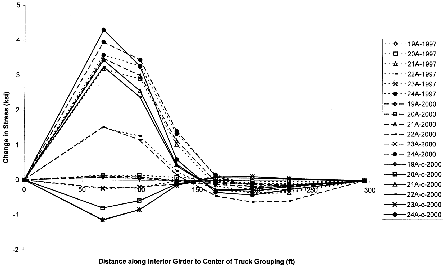
Figure F.103: Plot of Change in Stress with Nine Trucks 2000, Composite Analysis, N = 6 (Gages 19A-24A)
