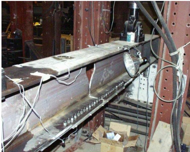
**Figure 3.5 Detail of Bolted Connection between Base Girder and Specimen**
