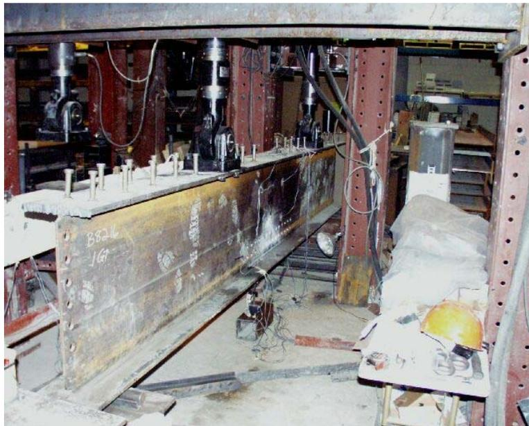
**Figure 3.10 Test Setup for Static Test on W27x94**
