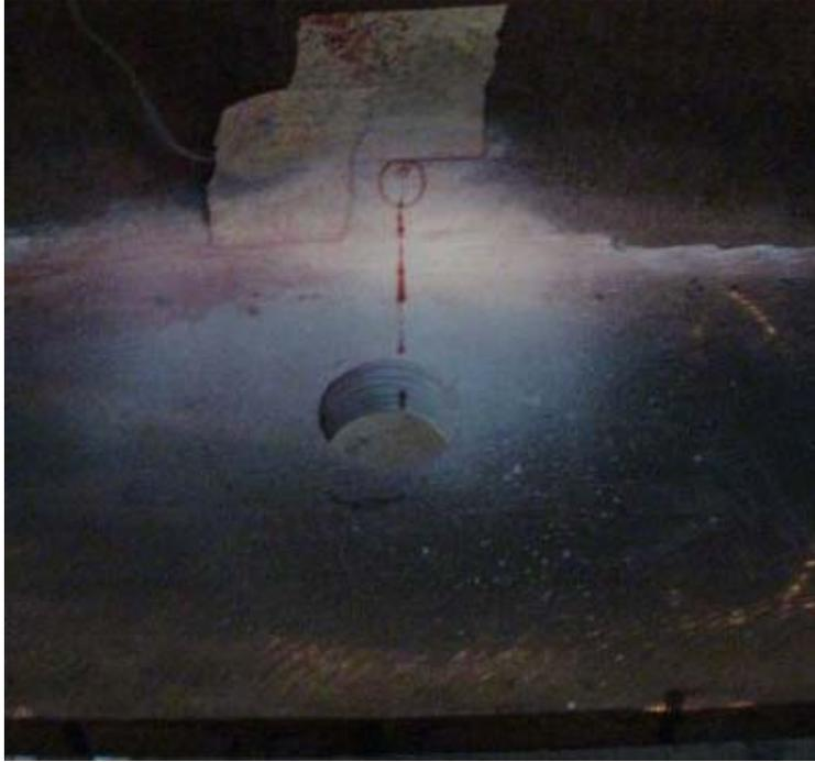
Figure 4.49 Crack Tip in Web (R-3-2)
