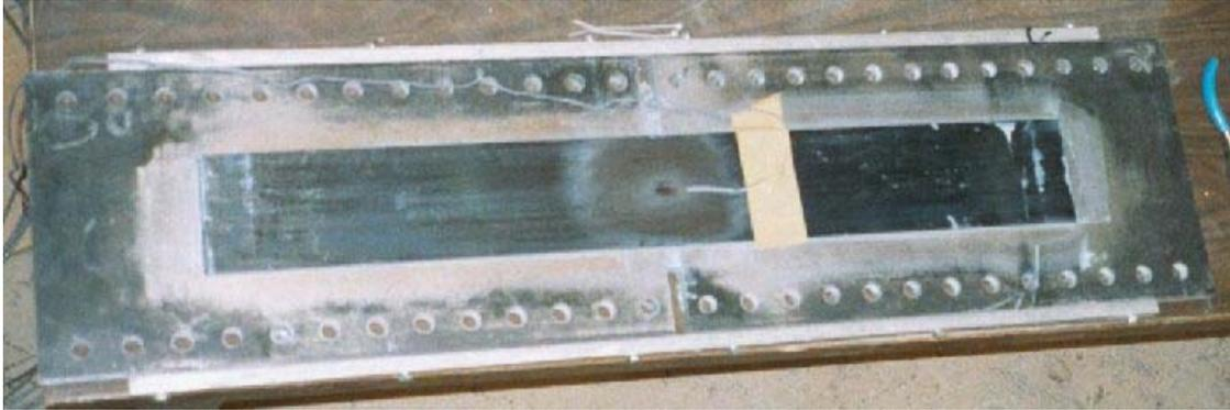
**Figure 3.4 Typical Specimen before being Bolted to W14x68 Girder - Specimen 1-2**
