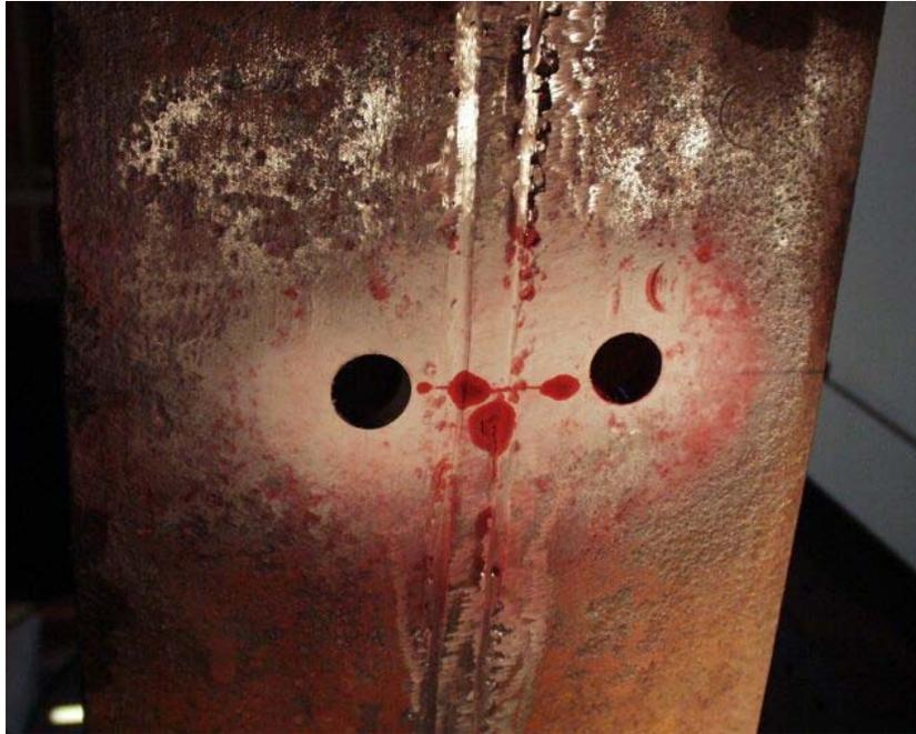
**Figure 4.37 Specimen with Crack and Holes (NR-3)**
