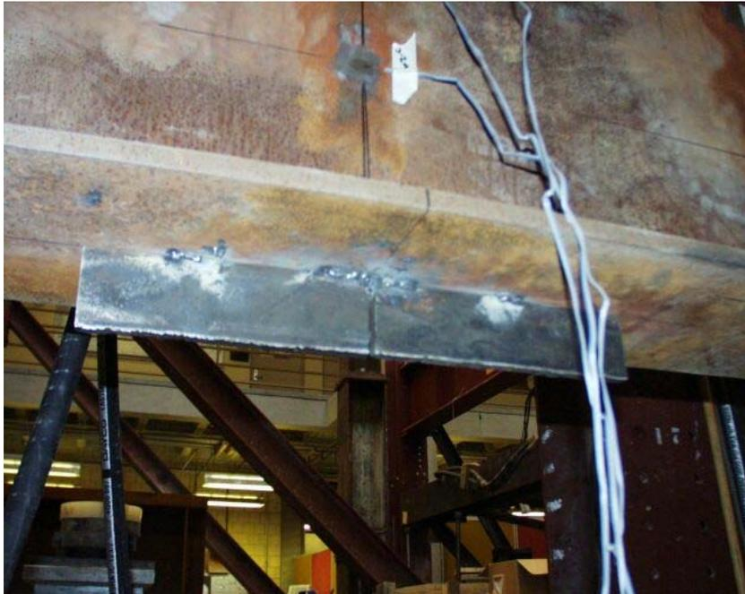
**Figure 4.36 Welded Steel Plates for Initiating Crack**
