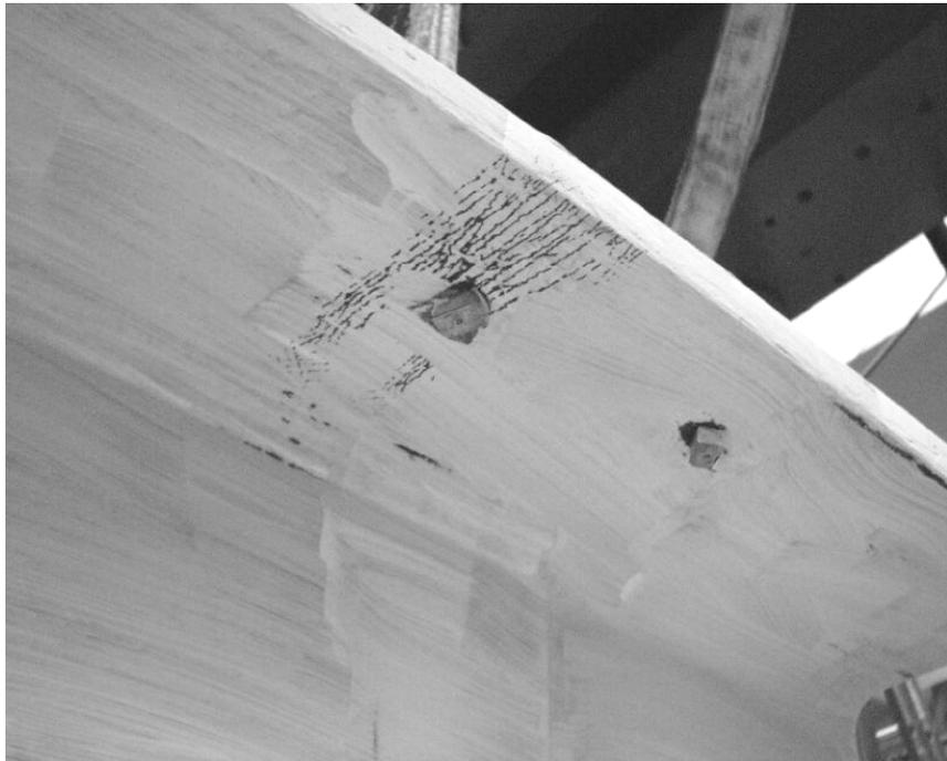
Figure 4.26: Yield Lines on Inside Face of Column Flange under Pull-Plate of Specimen 2-LFB
