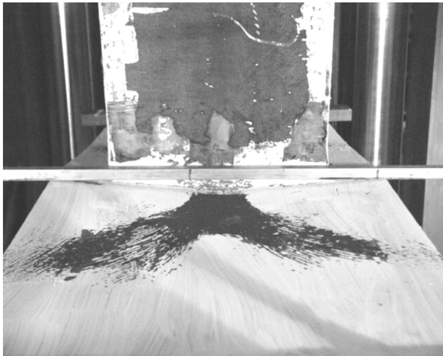
Figure 4.34: Specimen 1-LWY Flange Separation in Transverse Direction
