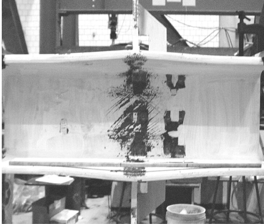
Figure 4.33: Specimen 1-LWY Flange Separation in Longitudinal Direction
