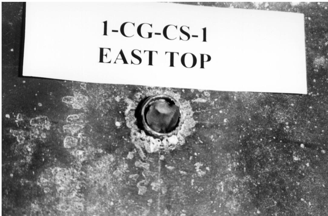
Figure 4.42 Photograph of stud failure surface for Specimen 8
