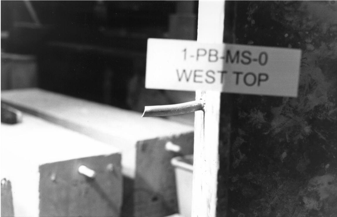
Figure 4.3 Deformed stud for Specimen 1
