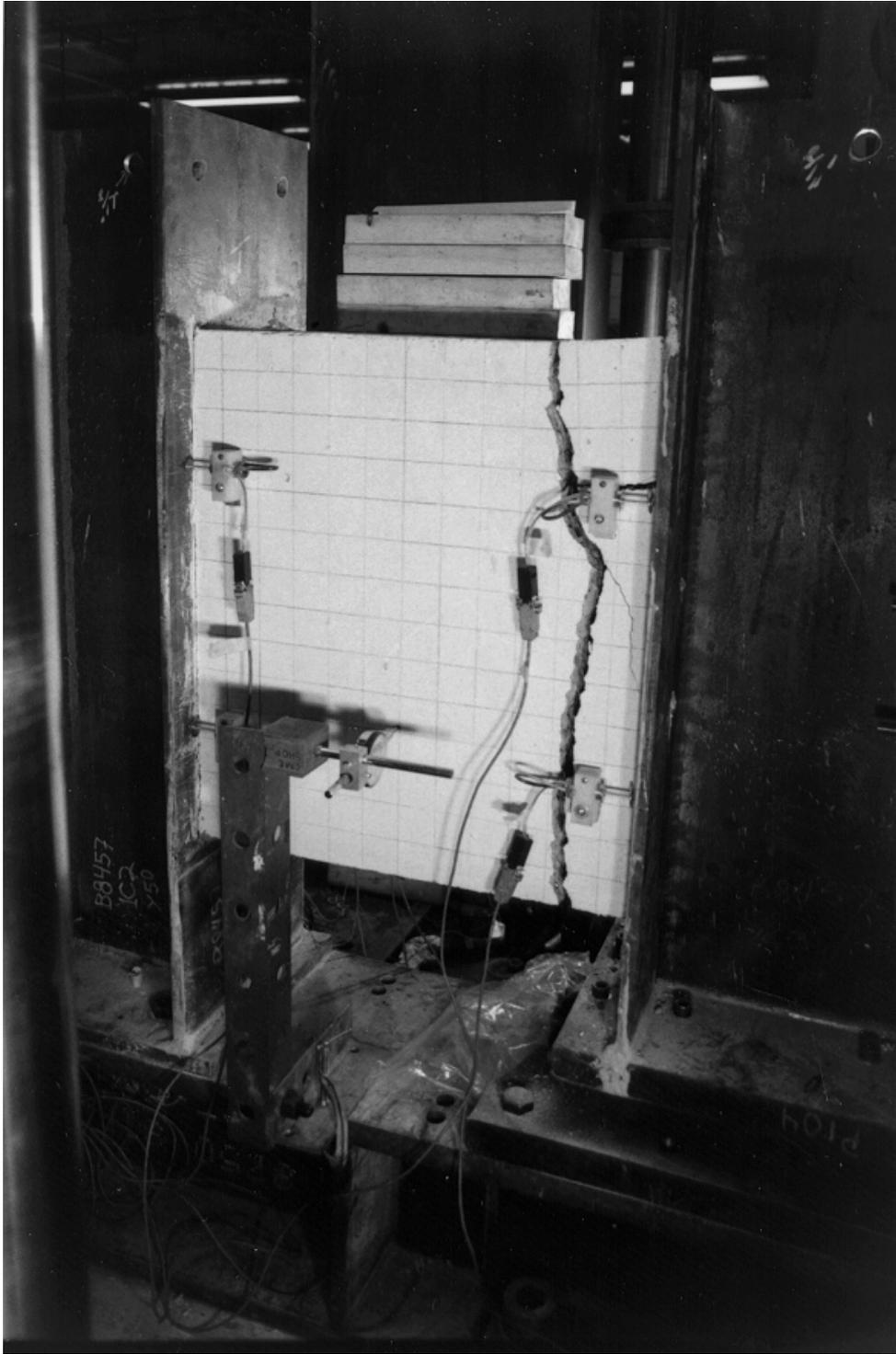
Figure 4.8 Photo of Specimen 2, north face, after testing
