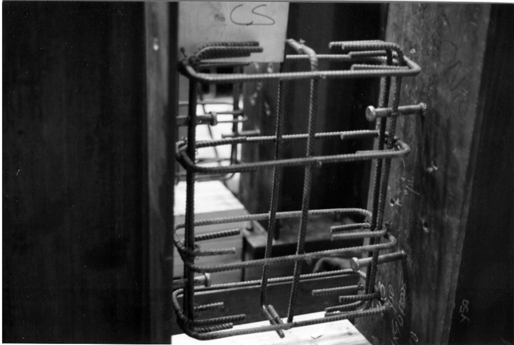
Figure 3.6 Photograph of the “Perimeter Bar” steel reinforcement configuration
