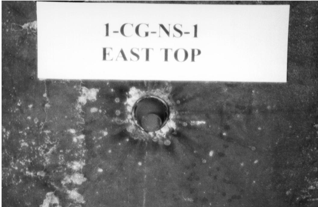
Figure 4.31 Photograph of stud failure surface for Specimen 6
