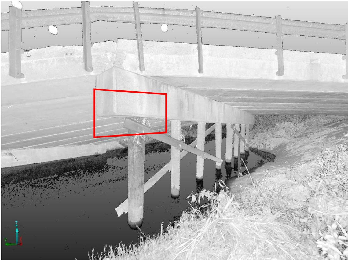
Figure 3.3: Scan data of testbed bridge with section utilized for data processing indicated.
