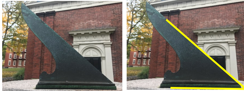
Figure 1. Photograph taken perpendicularly with respect to gnomon on sundial behind Holden Chapel at Harvard University (left) and yellow lines drawn on the photograph in order to measure the angle (right).
