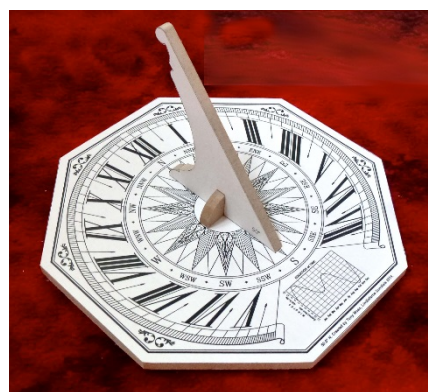
Figure 7. Hour lines and more precise time indicator lines on a horizontal sun dial with Equation of Time.
