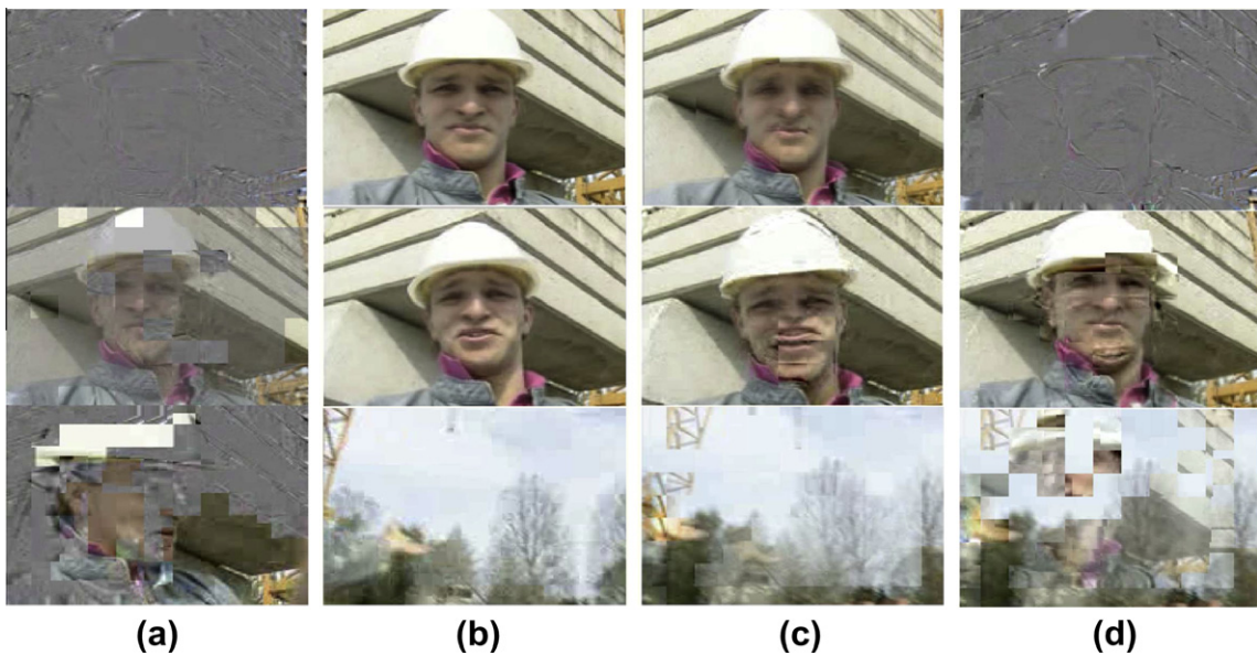
Fig. 6. Snapshots of foreman frame numbers 16, 160, and 305 while transmitted over WSNs in channel bit error rate 0.007 using (a) ARQ ( N = 4 ), (b) ARQ/RS/Erasure coding (4,106,4), (c) RS/Erasure coding (106,4), and (d) RS (106,100).
