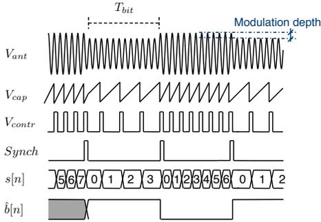
Fig. 3. Internal operation waveforms of the all-digital receiver.
