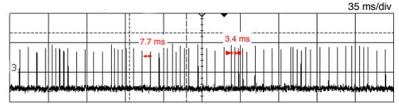
Fig. 4. Experimentally sensed output current of the energy harvester when receiving an input signal with powers  $P_0 = -9$  dBm and  $P_1 = -6$  dBm.
