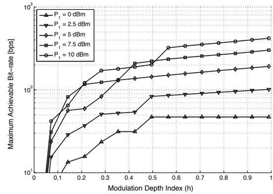
Fig. 6. Rate-energy trade-off of the proposed software-based receiver approach for SWIPT applications.
