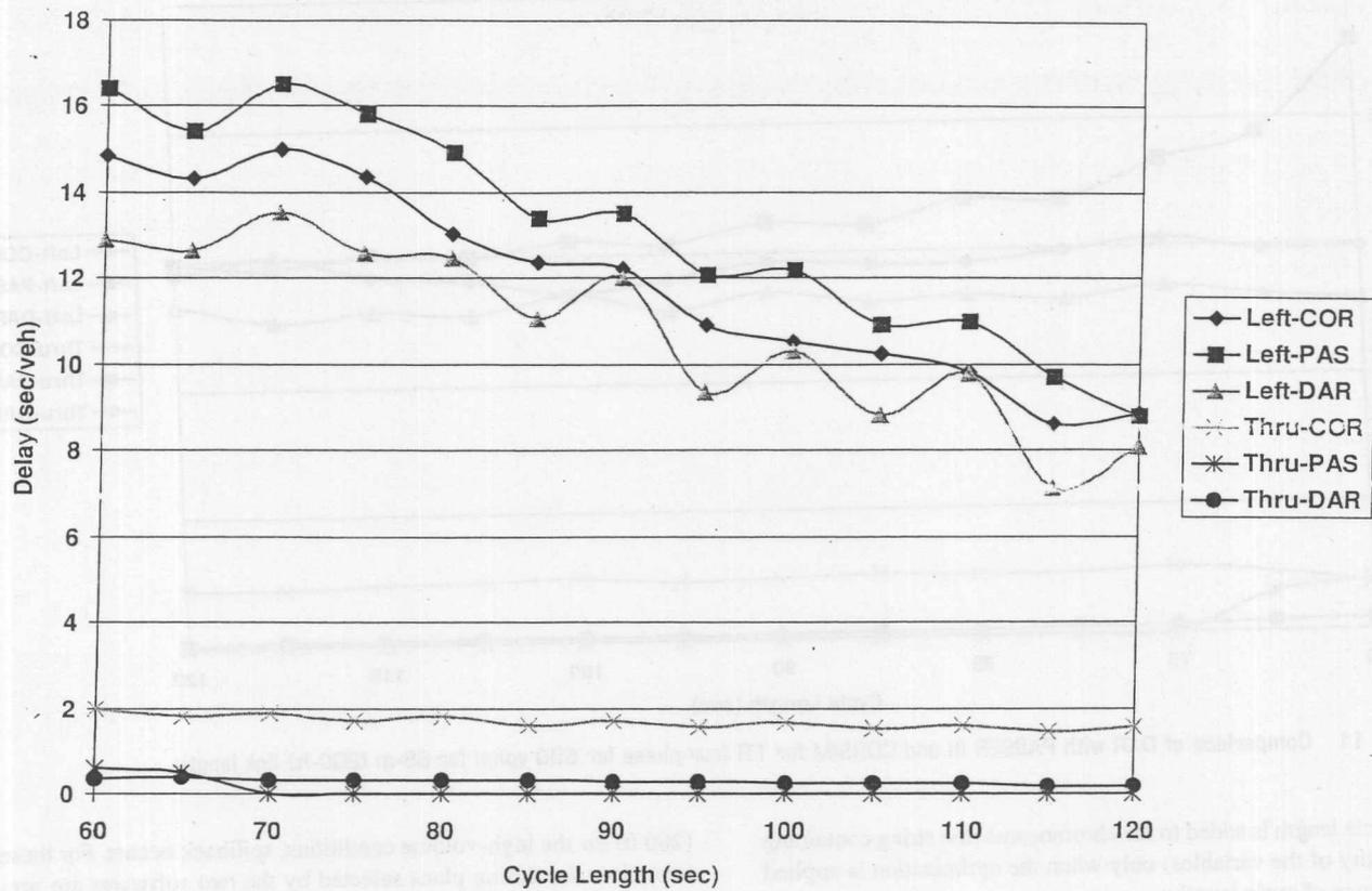
FIGURE 9 Comparison of DAR with PASSER III and CORSIM for TTI four-phase for 300 vphpl for 66-m (200-ft) link length.
