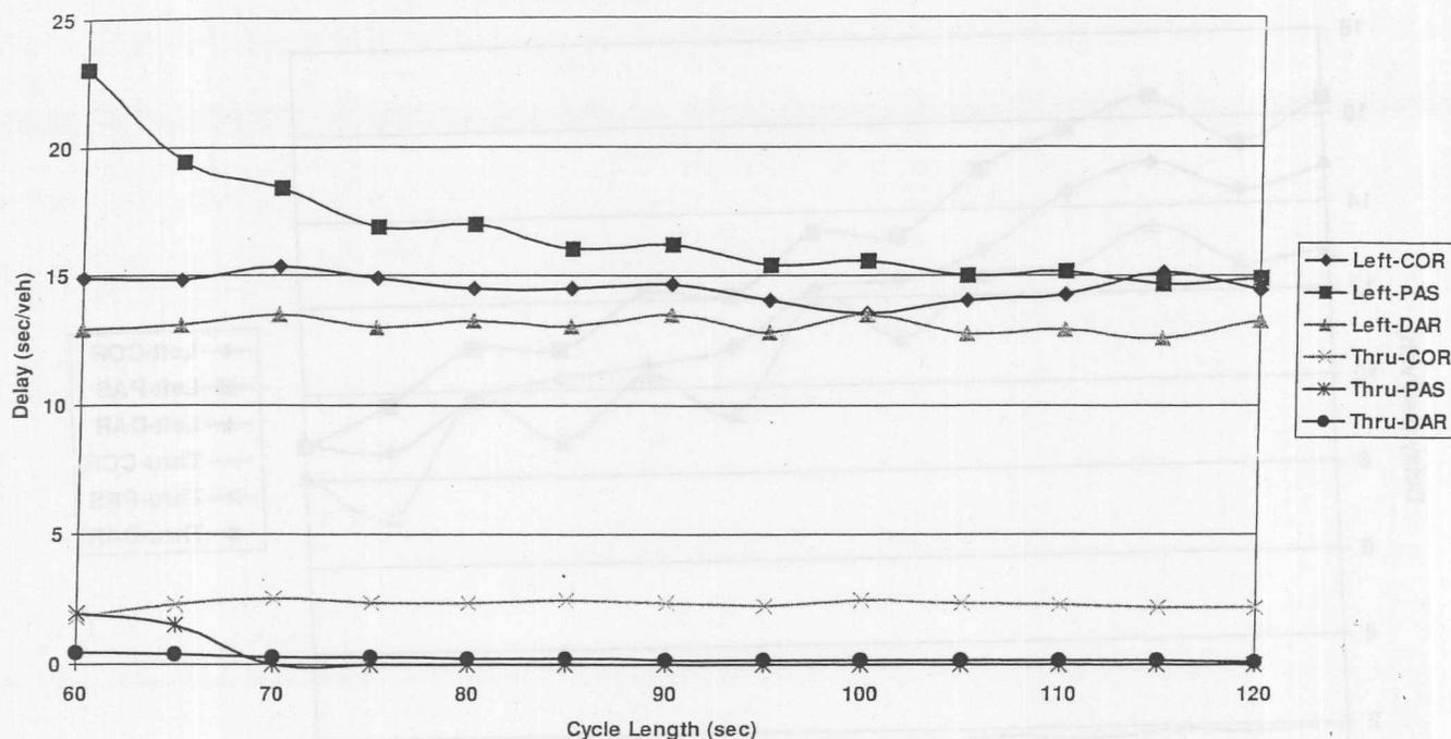
FIGURE 11 Comparison of DAR with PASSER III and CORSIM for TTI four-phase for 600 vphpl for 66-m (200-ft) link length.
