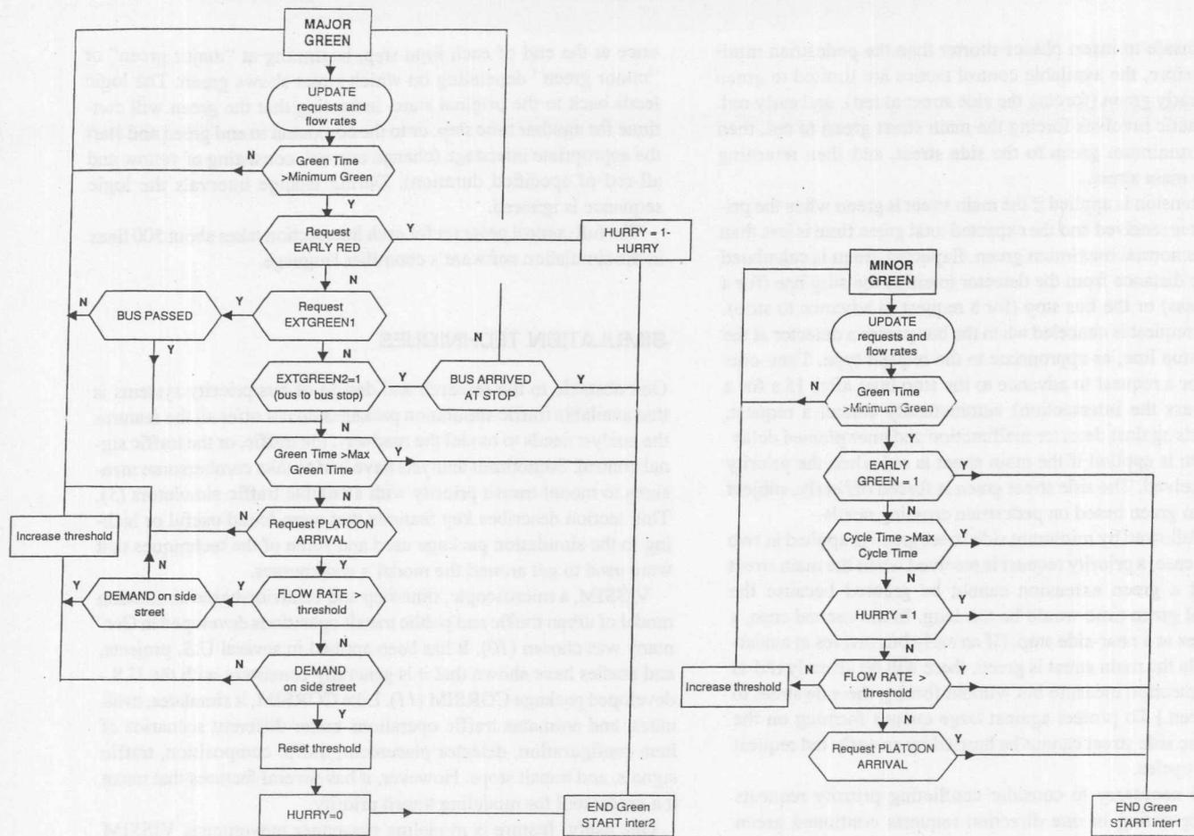
FIGURE 2 Traffic control logic.
