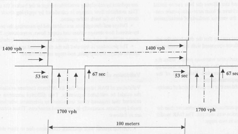
FIGURE 1 Arterial system with spillback conditions due to short downstream link (vph = vehicles per hour).
