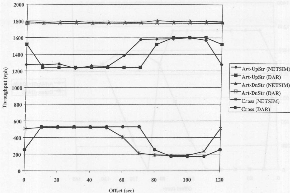
FIGURE 6 Throughput comparison for oversaturated link.
