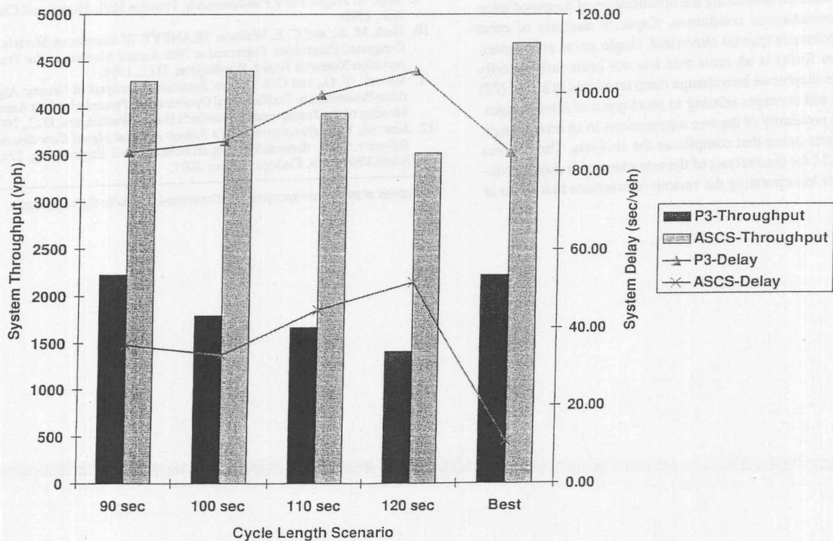
FIGURE 12 Comparison of optimal solution results of PASSER III and ASCS for 66-m (200 ft) spacing and 600 vphpl volumes.
