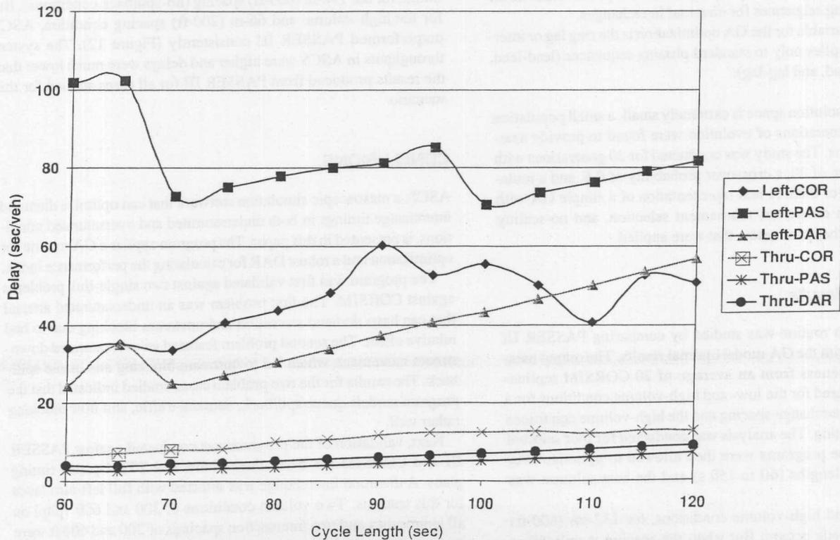
FIGURE 10 Comparison of DAR with PASSER III and CORSIM for basic three-phase for 600 vphpl for 66-m (200-ft) link length.
