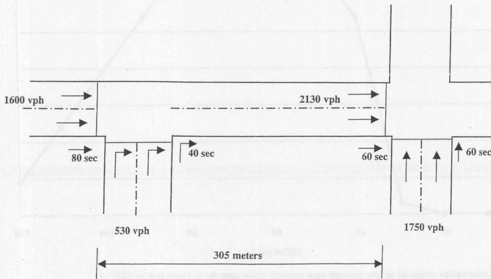
FIGURE 5 Arterial system with spillback conditions due to oversaturated downstream link.
