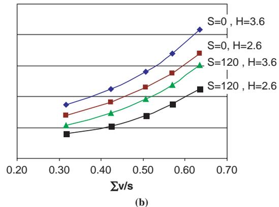
FIGURE 5 Expected cycle length as a function of demand, critical headway  $H$ , and detector setback  $S$ : (a) one through lane and (b) two through lanes.
