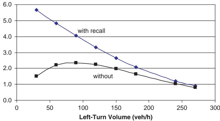
FIGURE 8 Minimum green lost time versus volume with and without recall.
