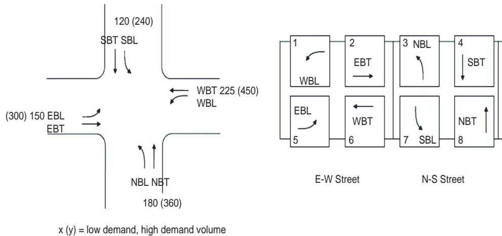
FIGURE 1 Example intersection with eight-phase dual-ring control (SBT = southbound through, SBL = southbound left, WBT = westbound through, WBL = westbound left, NBL = northbound left, NBT = northbound through, EBT = eastbound through, and EBL = eastbound left).
