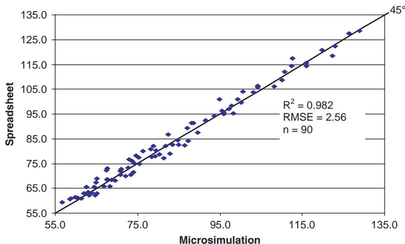
FIGURE 7 Expected cycle length for spreadsheet model versus simulation experiments.
