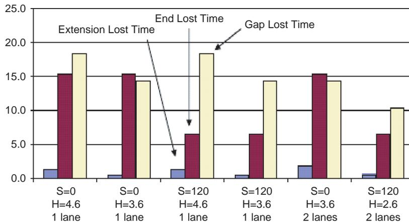
FIGURE 6 Selected lost time components per cycle as a function of critical headway  $H$  in seconds and detector setback  $S$  in feet.
