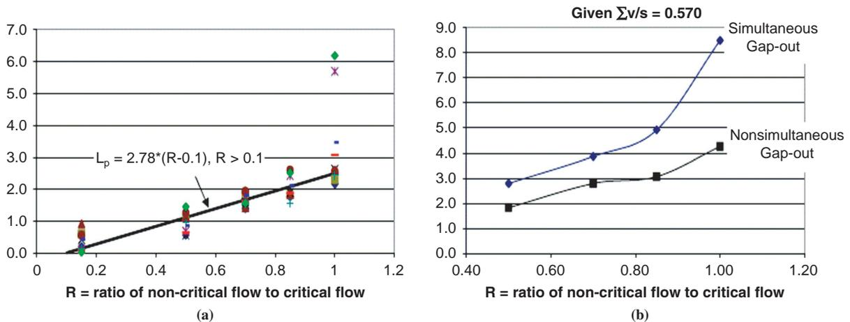
FIGURE 9 Lost time due to termination of green at barrier: (a) parallel extension lost time with nonsimultaneous gap-out and (b) sum of parallel extension or parallel discharge lost time and extension lost time.
