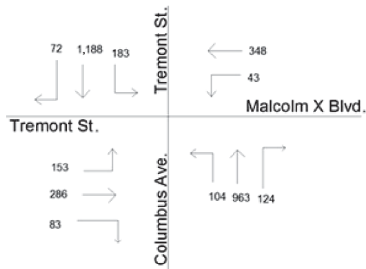
FIGURE 7 Turning movements at Roxbury Crossing (vehicles per hour, evening peak) (st. = street; ave. = avenue; blvd. = boulevard).
